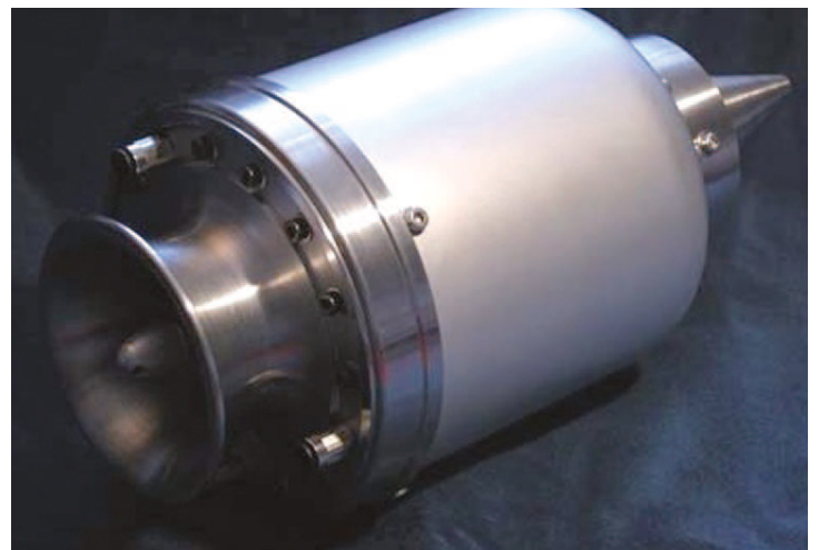
Figure 1. The model (left) and real prototype (above) of KJ 66 micro-turbine engine.
