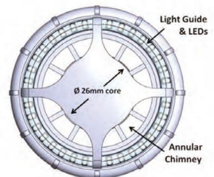
Figure 3. V3 Top View with Annular Chimney
