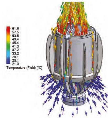
Figure 14. CFD Simulation of V8 Vertical Up Test
