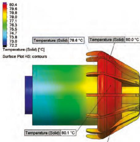
Figure 4. CFD Image of V3 Horizontal Position
