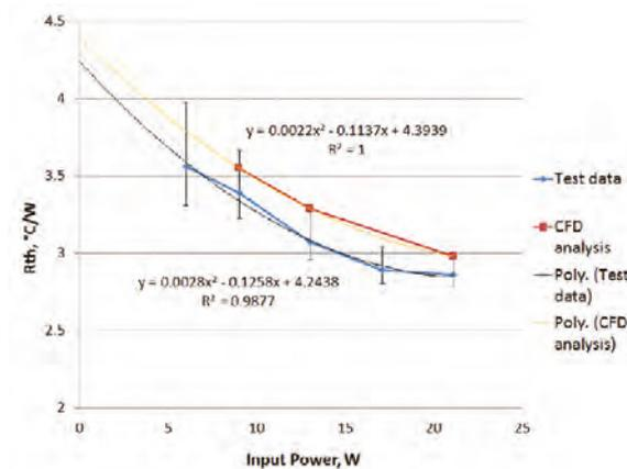
Figure 15. Performance of V8 in Vertical Up Orientation
