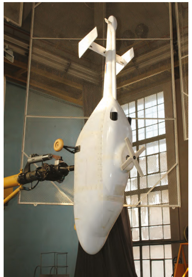
Figure 1. Light Helicopter model tests in wind tunnel T-105.
