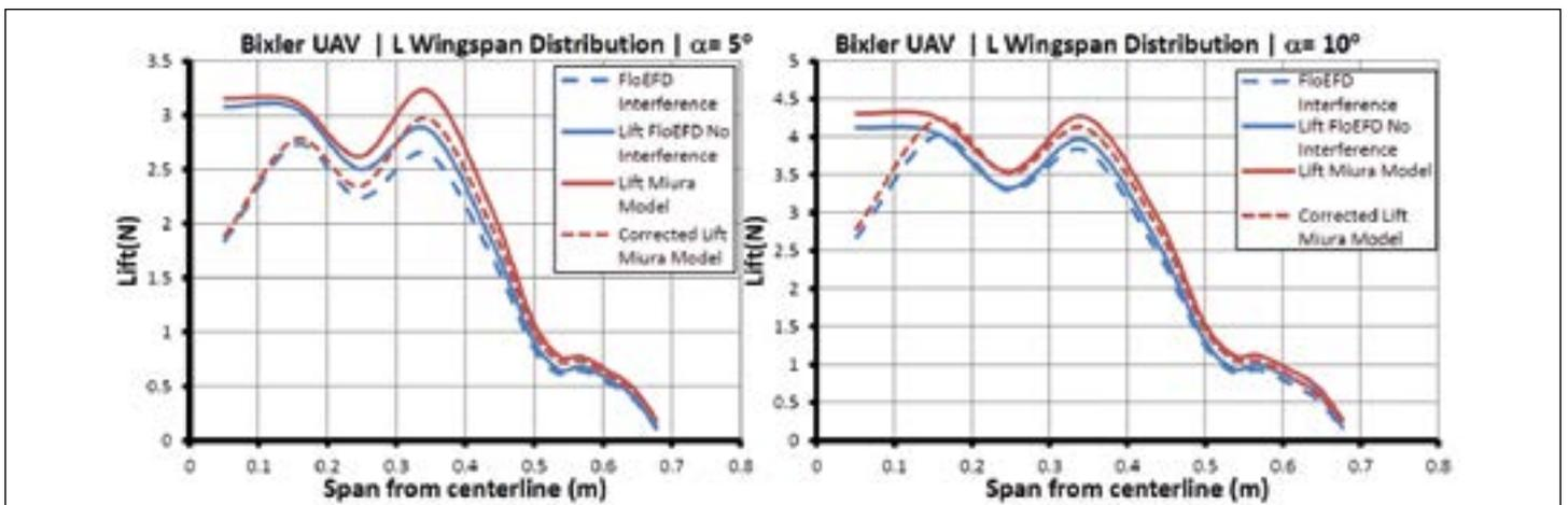
Figure 11. Spanwise lift and drag distribution with corrected and not corrected MIURA results compared to FloEFD results with and without interference
