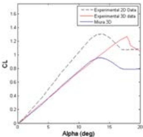
Figure 2. MIURA results without correction for stall prediction.
