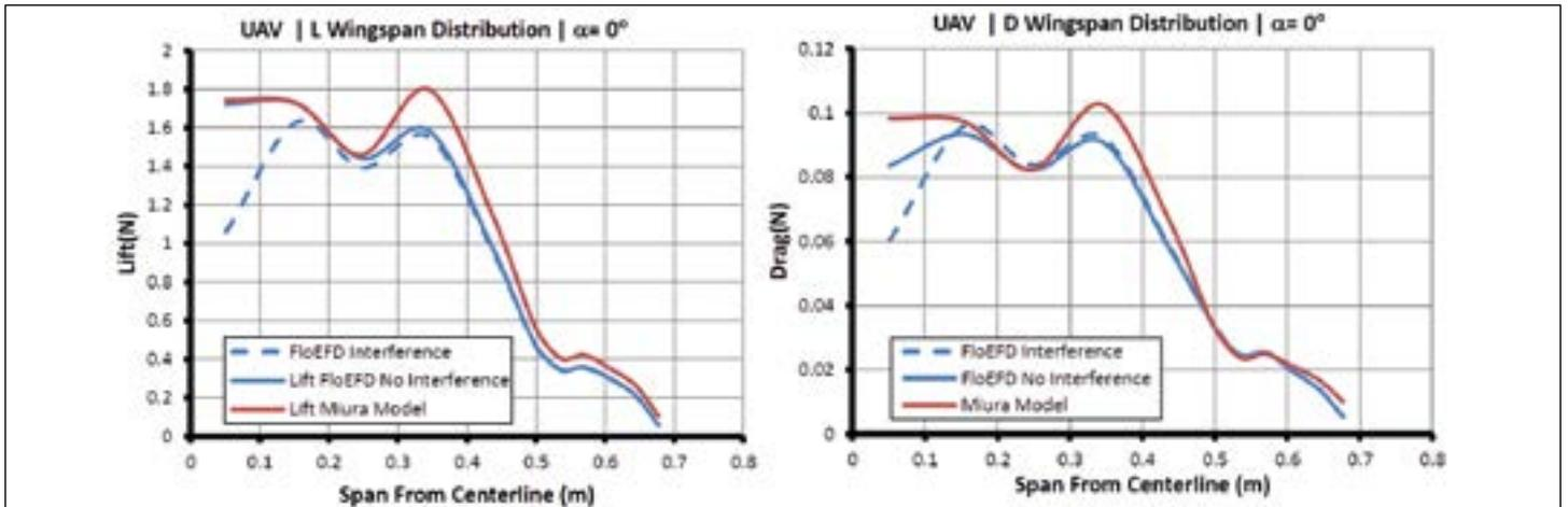
Figure 10. Spanwise lift and drag for not corrected MIURA results compared to FloEFD results with and without interference
