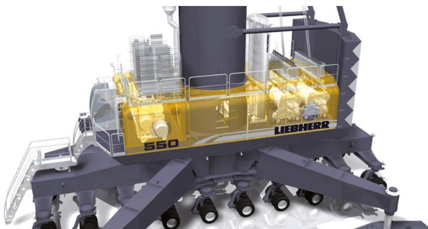
the engine hood, and typically include many devices such as cooler (diesel, water, air and oil), fans, exhausts, and hydraulics. This means that our CAD models can be rather large, with up to tens of thousands of components including all screws.
