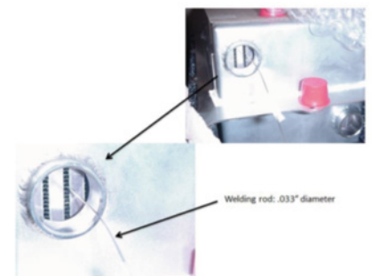
Figure 2. Fluid passage size at CAC entry
