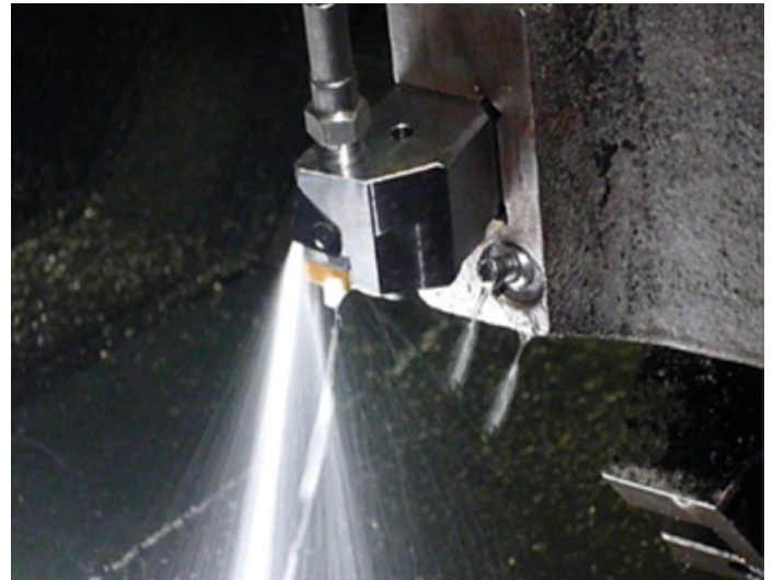
Figure 9. Final JT Holder Nozzle Spray Configuration
