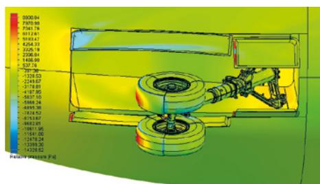
$\delta_{\text{strut}} = 60^\circ$ ,  $\delta_{\text{large door}} = 74^\circ$ ,
