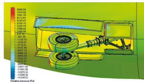
$\delta_{\text{strut}} = 45^\circ$ ,  $\delta_{\text{large door}} = 74^\circ$ ,
