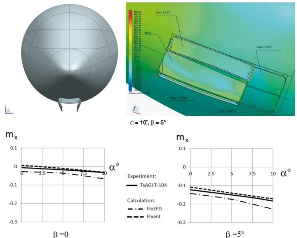
**Figure 4.** The model with opened large landing gear doors and the hinge moments of the large nose landing gear doors at  $\delta_{\text{door1}} = 60^\circ$ ,  $\delta_{\text{door2}} = 60^\circ$ ,  $\delta_{\text{strut}} = 0^\circ$  for the experiment,  $\delta_{\text{door1}} = 60^\circ$ ,  $\delta_{\text{door2}} = 0^\circ$ ,  $\delta_{\text{strut}} = 0^\circ$  for calculation,  $\beta = 0^\circ$  and  $\beta = 5^\circ$ .
