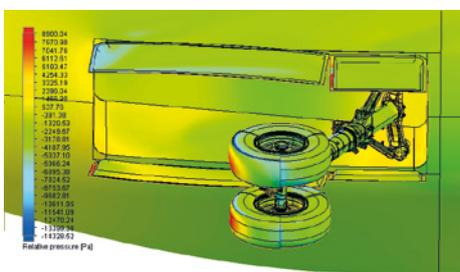
$\delta_{\text{strut}} = 75^\circ$ ,  $\delta_{\text{large door}} = 74^\circ$ ,
