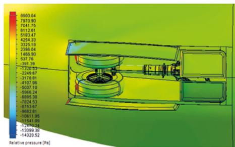
$\delta_{\text{strut}} = 15^\circ$ ,  $\delta_{\text{large door}} = 74^\circ$ ,
