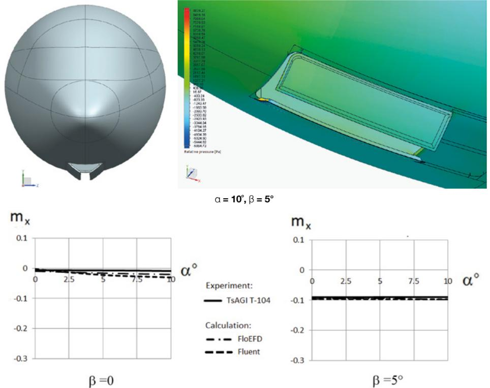
**Figure 3.** The model with the opened large landing gear doors and the hinge moments of the large nose landing gear doors at  $\delta_{\text{door1}} = 30^\circ$ ,  $\delta_{\text{door2}} = 30^\circ$ ,  $\delta_{\text{strut}} = 0^\circ$  for the experiment,  $\delta_{\text{door1}} = 30^\circ$ ,  $\delta_{\text{door2}} = 0^\circ$ ,  $\delta_{\text{strut}} = 0^\circ$  for the calculation,  $\beta = 0^\circ$  and  $\beta = 5^\circ$ .
