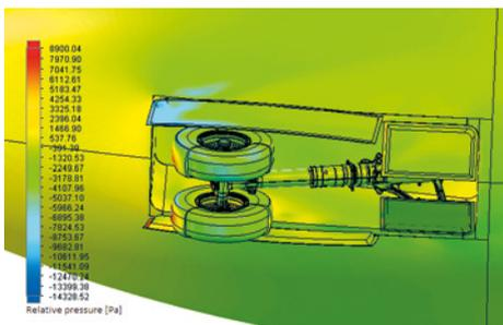
$\delta_{\text{strut}} = 30^\circ$ ,  $\delta_{\text{large door}} = 74^\circ$ ,
