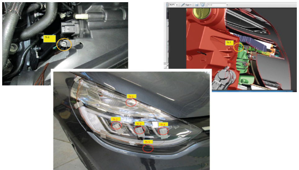
Figure 7: Location of the eight thermocouples for the Ambient Temperature Headlamp Engine Tests
