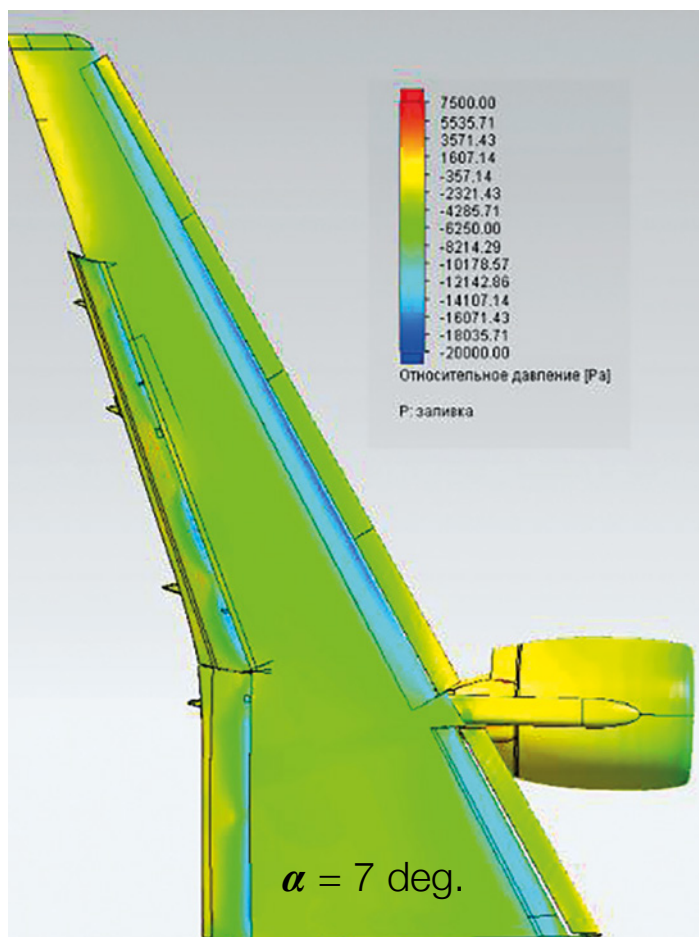
Figure 4. Computation Results: \Delta P on Wing Surface
